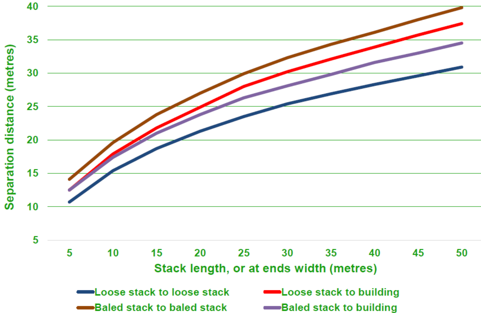
Graph 2. Stack lengths and separation distances plastic/rubber wastes (typical max burn 1,200 °C)
