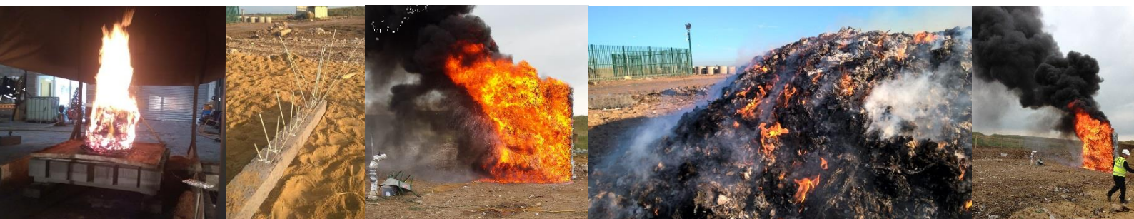
From left: Smaller scale laboratory burn tests, the 'porcupine' thermal sensor array used in larger scale stack burns, plastic bales burn test, RDF loose stack burn test, bale burn test general view.
